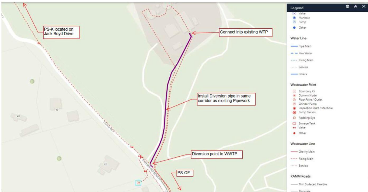
Figure 4-2: PS-K Diversion Alignment (Indicative Only) (WSP 2022)
